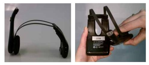
The dual headbands may become miss-shaped resulting in a loose fit. To tighten the "grip" of the headset, grab one side of the headset in each hand and pull the two sides past each other as illustrated in the photos.
