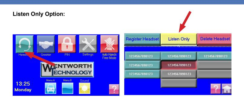
In order to prevent unintended communication between a headset and the order point, use the Listen Only Option, which disables the Center button but allows the Page button to function. When the headset is powered on or if the center button is pressed a voice prompt of "Listen Only Mode" is played to remind the user of limited operation.
