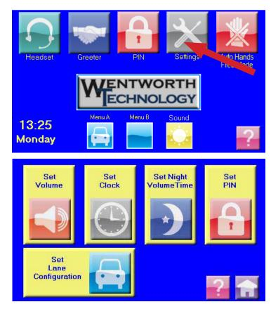
The "Settings" button provides access to the following five system settings categories: (1) Set Volume, (2) Set Clock, (3) Set Night Volume Time, (4) Set PIN, (5) Set Lane Configuration.
