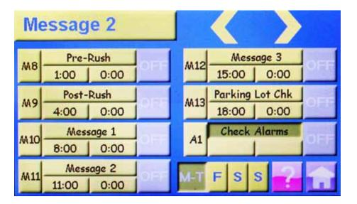
**Alerts:** The last option on MSG 2 is for ALERTS. An alert is a message that is repeated in the headset that is not activated based upon a time, but upon a switch activation. You may connect an infinite number of switches to the basestation in parallel. No matter which switch is activated, the same message will play.
