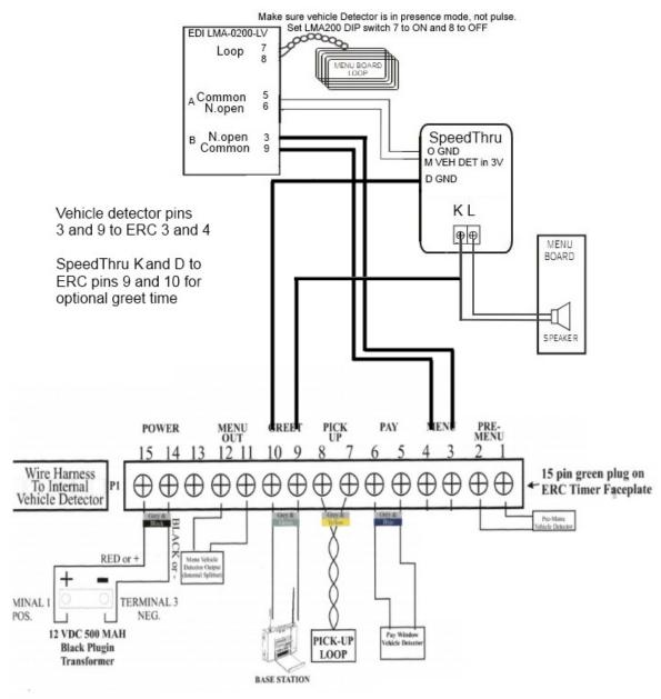
Make sure all wire to wire connections are soldered. Do not use wire nuts.
