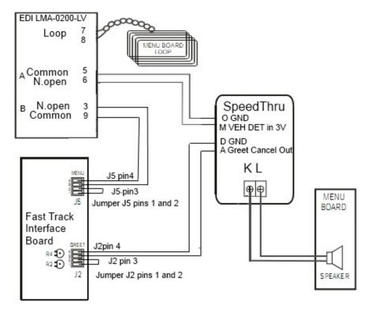
The Fast Track timer requires service window loop connections as well, these are not shown in this diagram. Refer to Fast Track timer installation instructions.
