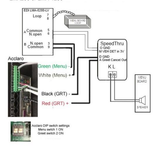
Make sure all wire to wire connections are soldered. Do not use wire nuts. All wire ends connected to terminal blocks must be tinned.
